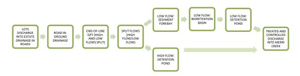
Figure 3.2. Proposed Stormwater Treatment Train
